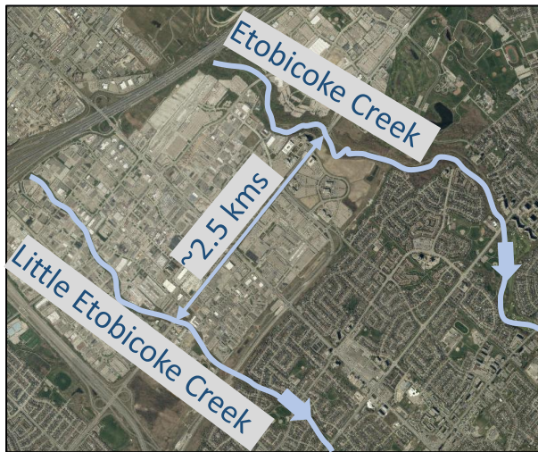
Alternative 1 – Flow Diversion to East
